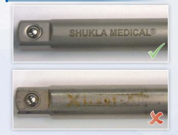
**Connection Threads Corrosion**
